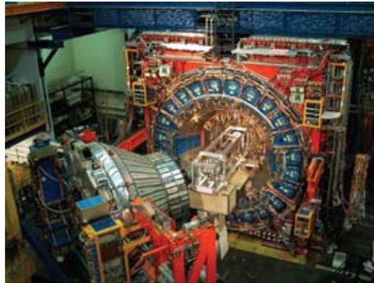
**Figure 1.** Picture of the CDF detector, as it was getting upgraded for the current run. The picture shows the new silicon vertex detector being installed inside the new drift chamber, both of which track charged particles. One of the new endplug calorimeters has been moved out to install the silicon detector.
