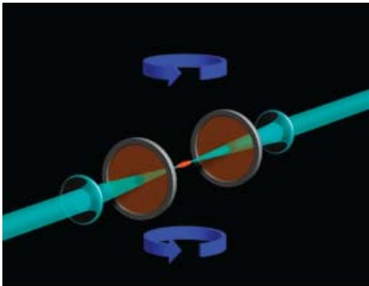
**Figure 1:**  $\text{CO}_2$  laser beam trap. Atoms are attracted to the focal point, forming a cigar-shaped cloud. Bias magnetic field coils (blue) tune the cloud to a collisional resonance.
